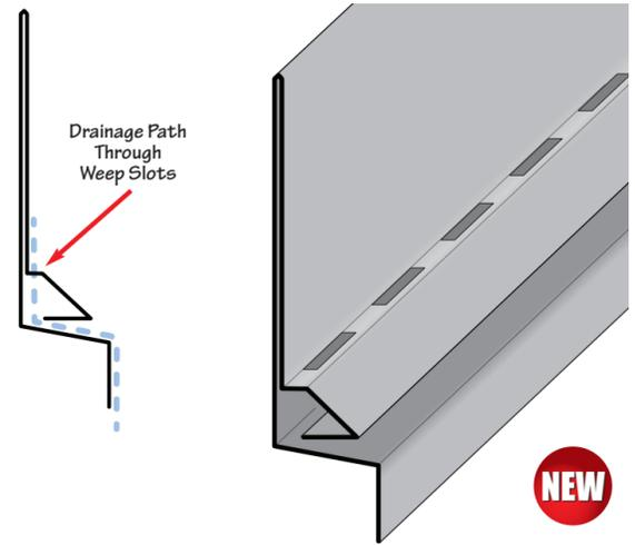
**TWWF: Tru-Weep™ Window Head Flashing**
